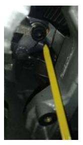
1. Make sure the Delete Kit is fitted on 2.5ltr engines with balance shafts removed. (Part Number ENG0298) use grease on O ring and retainer on the bolt with Snor washer.
