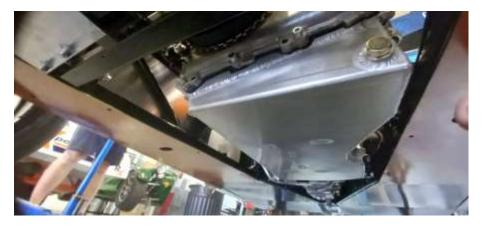
8. Go ahead and fit all other M8 by 25mm bolts with locking washers. Do not fully tighten. Let the sealant go off for 20 minutes or so before tightening all screws, start with the front edge M6 bolts – 11Nm then starting in the centre go opposites until all tight torque to 30 Nm. Then allow sealant to fully cure before filling with oil, ideally overnight / 24 hours. Also check that the sump bung is in place and tight with sealing washer.
